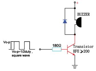
The base current lb should high enough so that it saturates the collector current of the transistor with the CB load.
